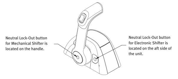
If your boat is equipped with Helm Master<sup>™</sup> there is a feature that is similar to a neutral lockout on other boats. When activated, the free throttle button allows opening the throttles on all engines without engaging the forward or reverse gear. The active indicator will be illuminated during operation.
